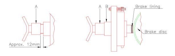
Brake released. Brake nut (A) screwed out approx. 12 mm. Brake operational. (A) screwed in to (B). The wind speed indicator is positioned on the operator's display.
